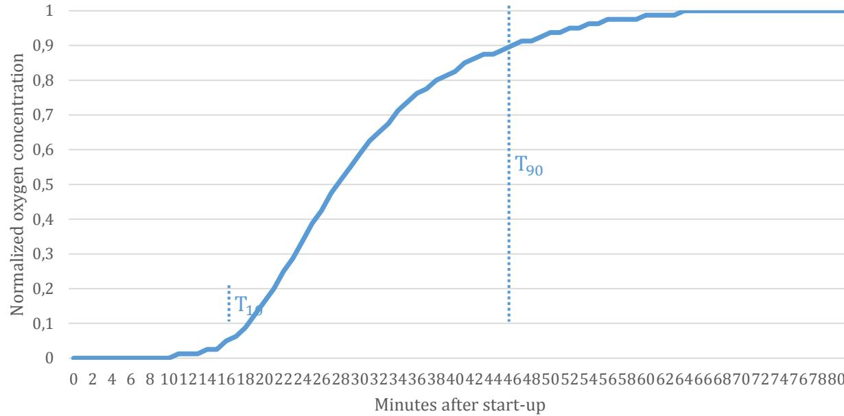
$$T_{10} = 19 \text{ min} \quad T_{90} = 46 \text{ min} \text{ at } 2000 \text{ m}^3/\text{h}$$
